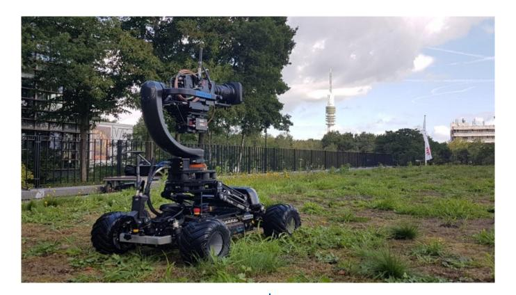
The AGITO has been developed as the only fully modular dolly system capable of working free roaming. Combining AGITO Sports with our V-Con Pro or Tower and our Shotover G1 enables complete freedom of movement.
