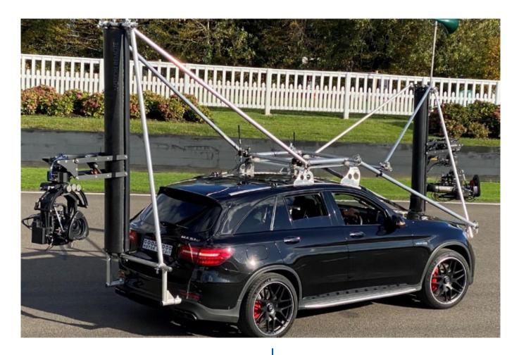
The Black-Tek Tower 24 is a vertical lifter for remoteheads and can be mounted on camera cars and or even used stationary. The Black-Tek Tower 24 can be used with smaller remoteheads like the Flighthead Mini 4 or Shotover G1 and is controlled by the camera operator via joystick or a foot pedal. The Black-Tek Tower 24 includes a shockabsorber to reduce unwanted vertical movement. With this shockabsorber, the total weigt of The Black-Tek Tower 24 comes to 34kg (75lbs).
