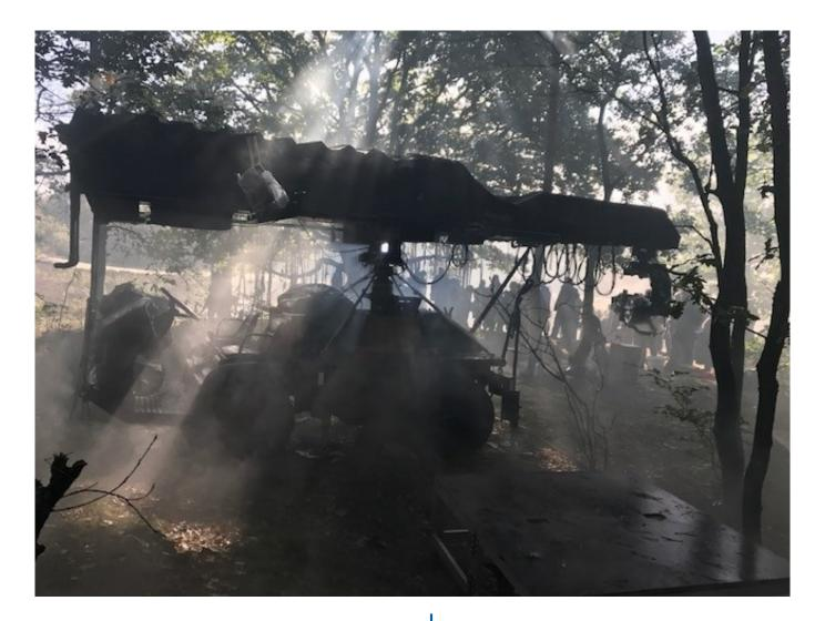
The Ectogator is a 4x4 off-road vehicle that simply takes the camera crane to the chosen recording location. Whether it be up hills, a muddy field or an isolated place. With its all-terrain tire sets and its heavy duty construction, the gator, and therefore also the camera crane, can be used in extreme conditions.
