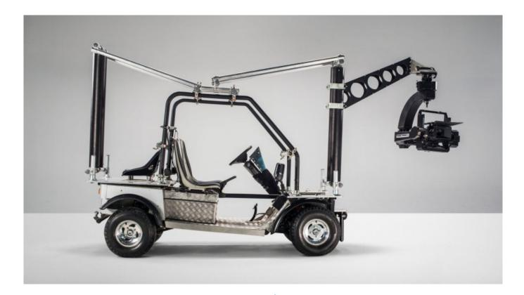
Vehicle designed for capturing moving scenes in locations where we need a quiet work atmosphere that respects the environment.lt is ideal for working in interios (recording studios, sports ...) and in public areas where it is not possible to set a vehicle with a combustion engine.
