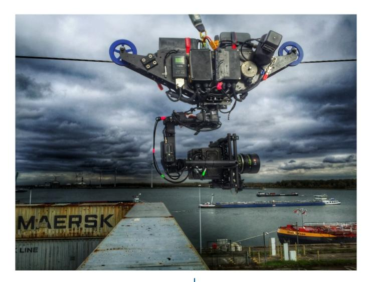
The Flyline is a cablecam system. And this by using two ropes, 1 to ride on and 1 as the safety. The Flyline does not require heavy winches. The Flyline makes use of a DC motor on the trolley along the cable. The power is provided by on-board lithium-polymer batteries. It is possible to reach speeds up to 45 mph (65 kph). The maximum rope length is 470 m at the moment.
