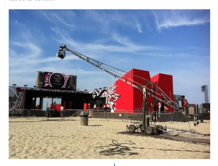
The GF 9 is a long elegant modular remote crane system. It reaches a maximum length of 9m by 1 meter intervals. You can easily determine the desired length on-site.
