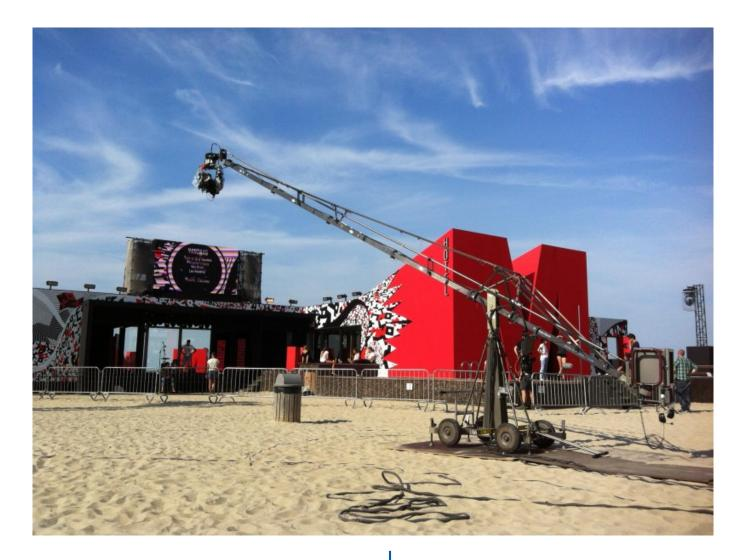
The GF 9 is a long elegant modular remote crane system. It reaches a maximum length of 9m by 1 meter intervals. You can easily determine the desired length on-site.
