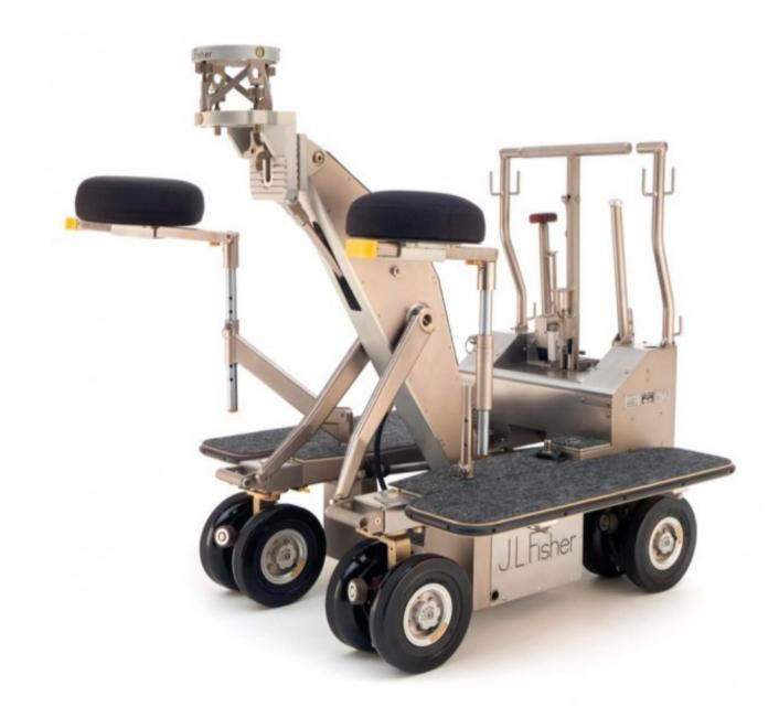
This is the smallest Fisher dolly, compact "lightweight" and maneuverable. The Dolly 11 has similar characteristics and operating as Dolly 10. This Fisher dolly is designed and produced to meet the demands of both the film and television industry. The compact size, the three-way control and the very stable lift arm provides a wide and flexible deployment. The Fisher dolly is reliable, quiet, smooth in operation and secure.
