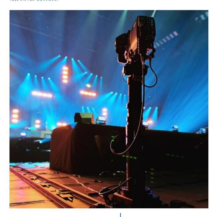
The Junior is a wireless compact dolly that can be remotely operated. A telescopic column adds a perfectly stable motorized vertical axis. Precise mechanical engineering and proprietary motor drives allow the junior to embark up to a 160mm lens HDTV lens with perfect stability.
