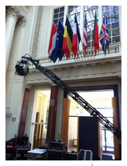
The Maxi-Jib is a classic light studio crane. It's ideal for smaller studio settings. The arm can be built in different lengths between 1.50 m and 4.60 m. The Maxi-Jib is light, slim and easily movable without compromising stability. The Maxi-Jib can be mounted on different dollies and can be equipped with most remote heads.
