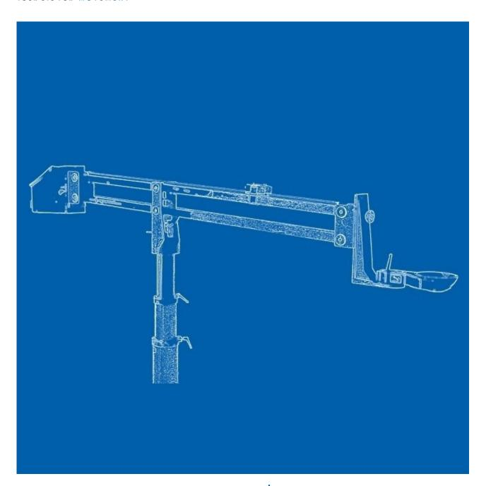
The mini-Jib is a jib-arm used in EFP recordings. Either a 100mm bowl as a 150mm bowl can be used.
