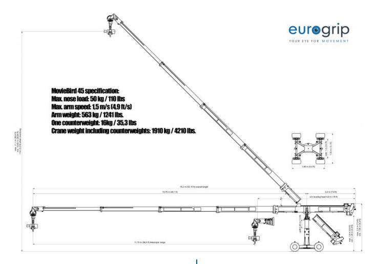
The Moviebird45 is a versatile telescopic crane suitable for any film set or TV studio. The crane is universal in use and depending on the weight of the camera package, it is possible to change the length and bring the reach from the arm from 35 ft to 45 ft (10,67m to 13,72 m) in a few seconds. The Moviebird45 is the most favorite telescopic crane on the market today.
