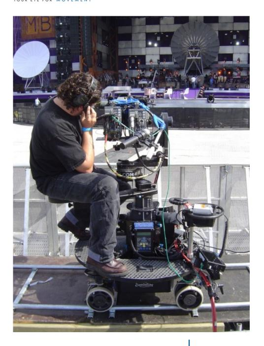
The Panther Evolution is the standard among film dollies. The hydraulic column operates very smooth and delivers maximum stability. High-end wheels and PDC tracks provide the most stable travel-shots. Accessories like snake, low-bowl, U-Bangi, low-base platform, risers and super-jib II are all available to make the most extreme shots. The arms are retractable, to operate in very tight spots. On a studio-floor you can use this dolly on hard wheels, switchable between 2 and 4-wheel steering.
