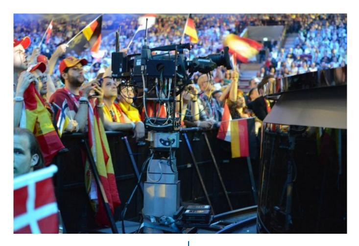
The Sam-Dolly is our self-developed travel-cam. It is suitable for all common travel-shots, even completely wireless if desired (for example on a fully enclosed circular track).
