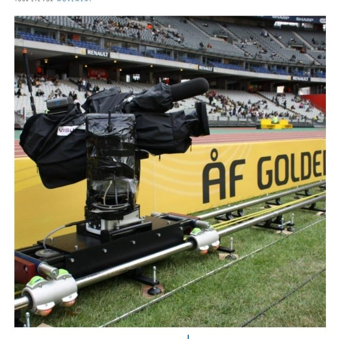
The Speedcam is a super fast travel-cam. This wireless application is mainly used for athletics in the track venues. So far we covered the Diamond League in Paris and Brussels. The Speedcam is developed by Eurogrip!
