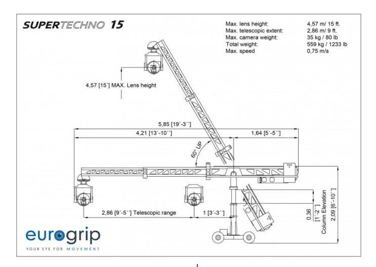
The (r)evolution on using cranes in small spaces. Enables you to perform complex camera movements between obstacles that previously were not possible.
