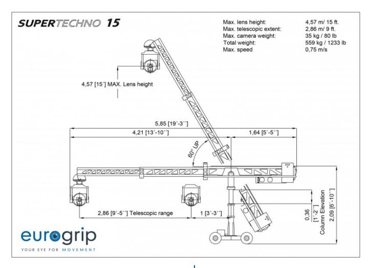
The (r)evolution on using cranes in small spaces. Enables you to perform complex camera movements between obstacles that previously were not possible.
