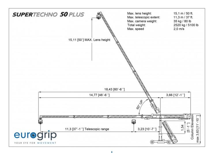
This giant has more than 14 meters of telescopic crane length combined with an enormous speed and stability. This techno is the ultimate tool for those who want to achieve complex crane movements of the highest level. The potential of this high-tech device is nearly infinite.
