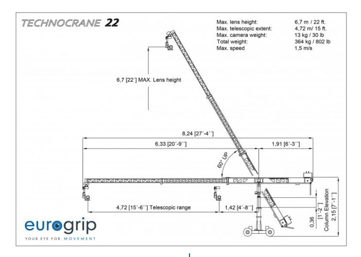
This is the lighter version of the standard Super Techno 22, but with its maximum length of over 6 meters it is one of the most used cranes in small or medium television-sets for the moment.
