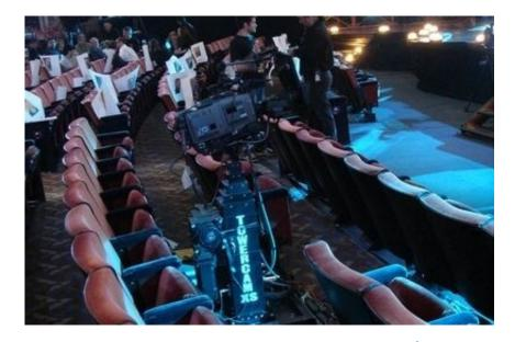
The TOWERCAM XS+ is the smallest version of the TOWERCAM. The minimum lensheight of 1,25 m and a lift of 1,3 m allows a camera movement with discreet technology.
