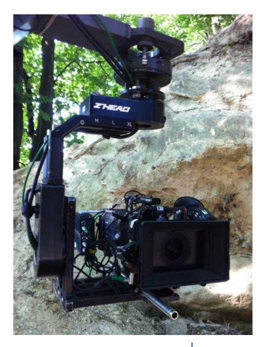
This head that hangs by default under the Super Technocranes, can support almost every camera (both video and film) and is fully modular. It can be built with 2 or 3 axes, in different sizes.
