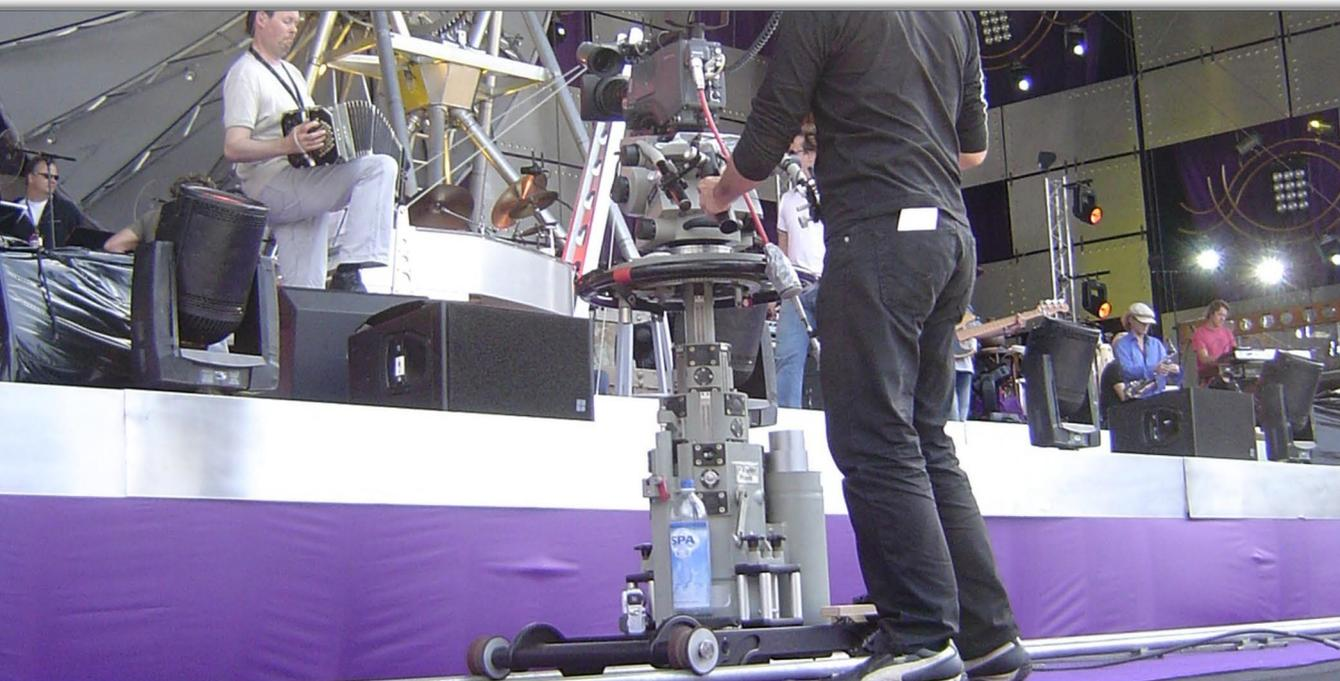
The Plover-Dolly is the ideal solution to adapt a studio camera with his own pedestal column on a travel track. Both Osprey, Osprey Elite, Pedestal as Teal can be fitted on this dolly in a few minutes. The camera operator can make smooth travel-shots, with long lenses using very little strength.
