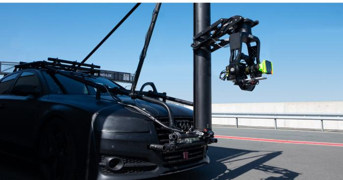
The Tower 24 is a vertical Lifter for Remoteheads and can be mounted on camera cars and or even used stationary. The Tower can be used in conjunction with our Flighthead Mini V4 and V5 and controlled by the camera operator via joystick or foot pedal. The Tower is available to rent separately with a driver and technician as well as a full package which includes the Porsche Cayenne and equipment as listed below.
